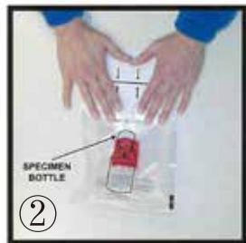
Figure 2: shows the specimen at the bottom of the bag and the area above the specimen being flattened in preparation for the adhesive tape to fold over.
