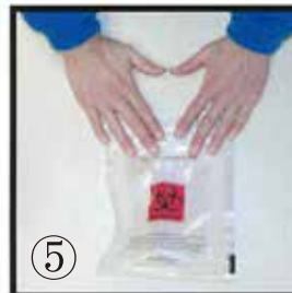
Figure 5: shows the middle finger of both hands being used to press the adhesive together. Start at the center of the fold and work outward. Please be sure to firmly press the entire adhesive area, especially the folded edge and corners. PRESS FIRMLY AT THE CORNER AREAS INDICATED BY THE ARROWS.
